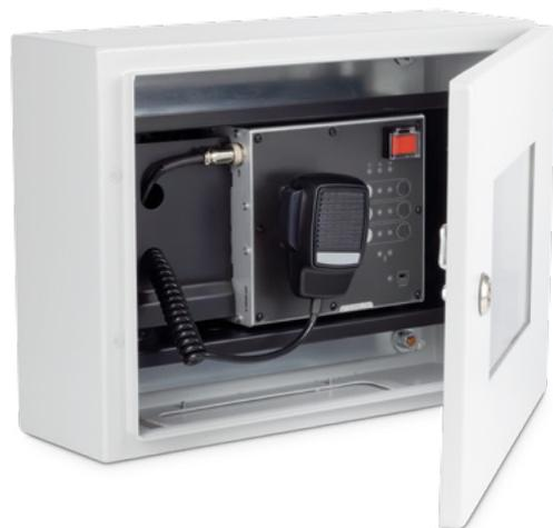
The ABT-DFMS-A PP is a monitored emergency microphone unit designed to operate a platform announcement point. The device connects to the core paging system via TCP/IP network, using either copper or redundant fibre optic interface. The ABT-DFMS-A PP can be used to make live broadcasts to pre-programmed zones or zone groups. It shall also allow to trigger alarm mode and broadcast pre-recorded messages from the
