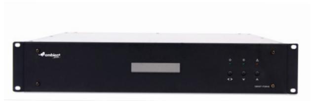
SMART-PSM48/E Power Supply Manager is designed for distribution of DC Power Supply from Power Supply Units (PSU) and a back-up battery. The unit controls battery charging and distributes power supply to all Voice Evacuation System (VES) equipment at max. 60 A. When the system uses battery back-up, the power supplied is 3.2 kW (48 V).
