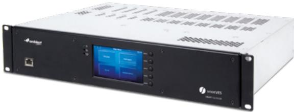
SMART-CU-11LT Control Unit (CU) is a matrix mixer of input signals which it routes to 4 100 V internal audio buses, a 45-channel digital system buses or directly to audio outputs in a unit. SMART-CU-11LT is designed to work for small PA and VE systems or as an extension unit in more complex systems.
