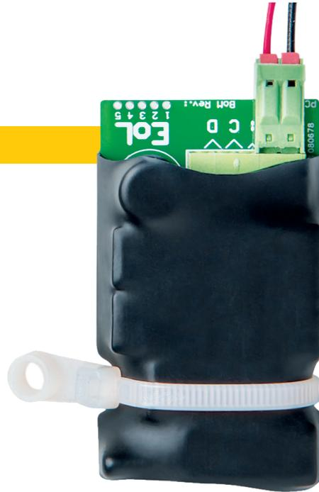
ABT-EOL monitors the integrity of a loudspeaker line and all of its branches. Supervision of branched lines requires EOL module for each branch. ABT-EOL provides a filtered load exclusively at the pilot tone frequency and increases reliability of loudspeaker surveillance method based on impedance measurement. Module connects
